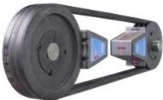
Both units facing each other in the pulley grooves
