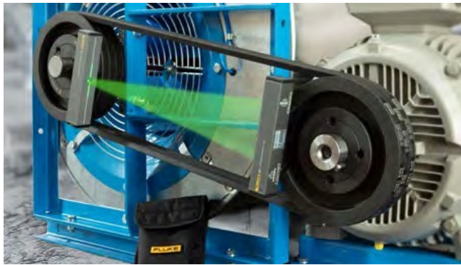
Fluke 835 laser line across a belt drive
