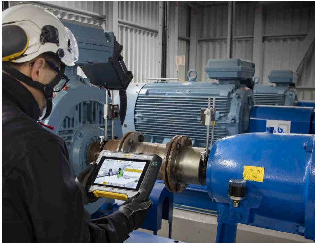
Laser system set up on a motor-driven machine
