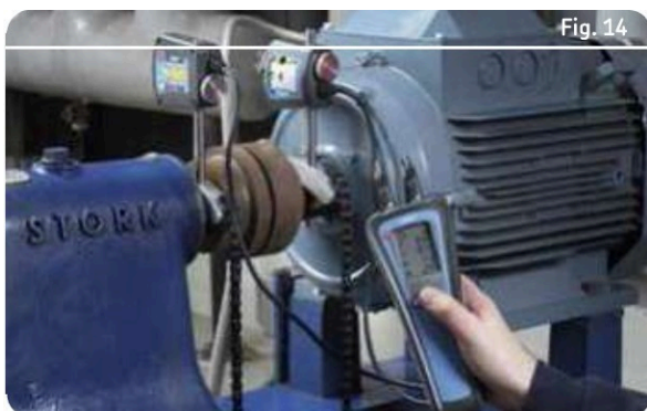
A laser tool measuring shafts on a motor
