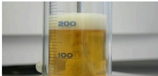
Foam on the surface does not disturb a hydrostatic reading
