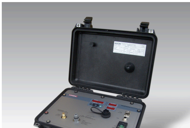
Analyzer in its case: display, pump switch, INLET and OUTLET ports
