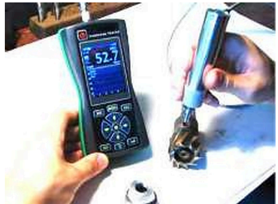
UCI test on a hardened part
