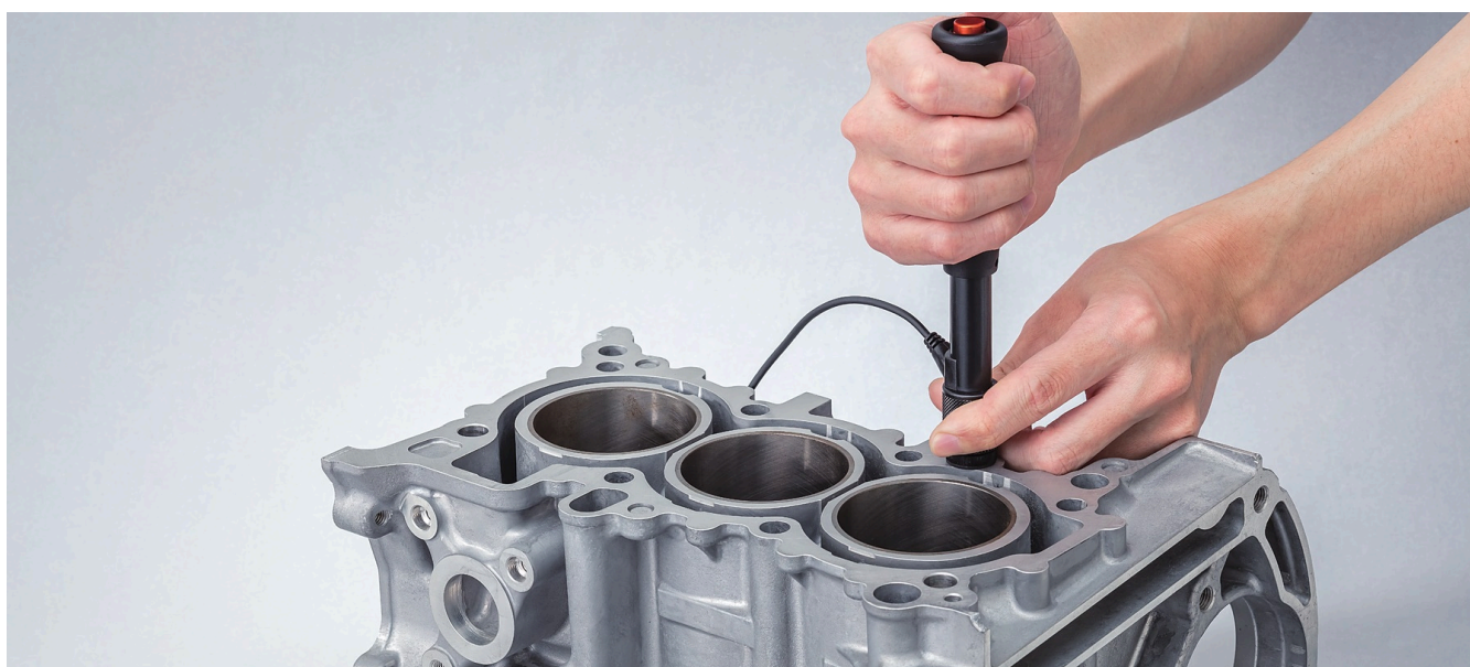
Hand-held rebound test on a large casting
