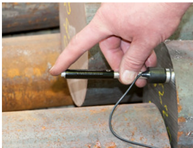
Rebound test on a large shaft
