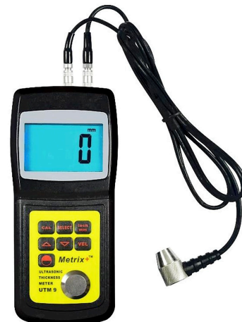
Basic gauge, twin-lead probe
